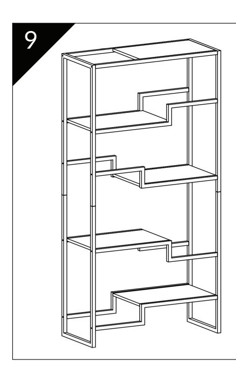
Place into position. If unstable, adjust feet levelers. To install anti-tipping wall mount, proceed to step 10.
