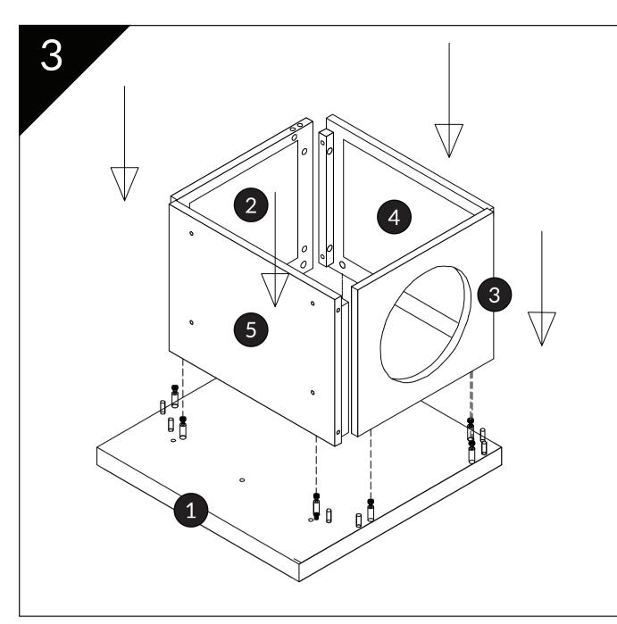
Place parts 2, 3, 4, 5 over installed hardware on part 1.
